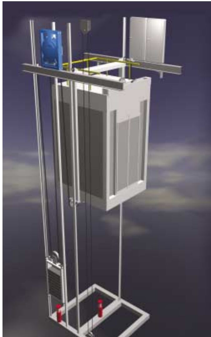
Machine-Room-Less Elevator (Roof Top Mounted Type)
